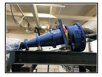
The facility had a cyclone separator which uses gravity to remove lighter materials from the top and heavier materials from the bottom.
