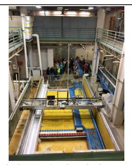
Ali and Lindsey gave AEG members and students a tour of the University of South Carolina's hydraulics lab and explained how they set up large scale dam and levee breach models.
