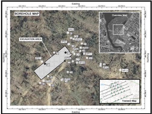
Exhibit 1: MIP and vertical profile sampling locations. The vertical profile locations were located along six transects displayed in the box in the lower right-hand corner.
