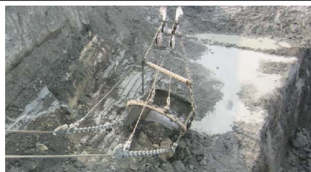
Figure 3. View from the operator's seat. Drag line bucket is exposing the phosphate ore (tabular feature).
