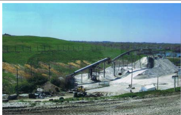
Taken from Southside Sanitary Landfill, Indianapolis, IN; the entrance to the Martin Marietta underground mine and the conveyor belts bringing aggregate out of it is in the foreground, the grassed-over landfill wraps around and can be seen in the background.
